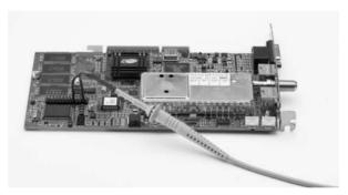
The 2.5 to 2 mm banana plug adapter provides a way to easily connect the probe signal input to a standard 2 mm banana jack. All outer surfaces are non-conducting to minimize shorting hazards.
